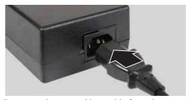
3 To disconnect the power/data cable from the power module, press inward on the two connector latches, then pull the plug away from the module.
